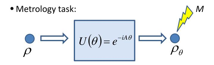
The basic task is to estimate the parameter  $\theta$  in the dynamics. In order to measure  $\theta$  we prepare a probe state  $\rho$ , let it evolve, and finally measure the evolved state with an operator *M*.
